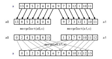
Figure 11.1: The execution of mergeSort(a, c)
